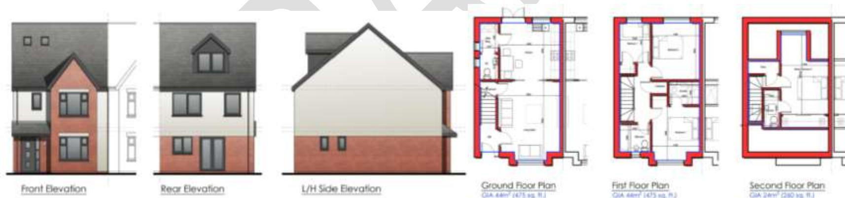
4.6 As the elevations illustrate, House type A will be a mix of red brown facing brickwork to the lower level with painted render above, under a synthetic slate roof. Windows and doors will be grey upvc double glazed units.
